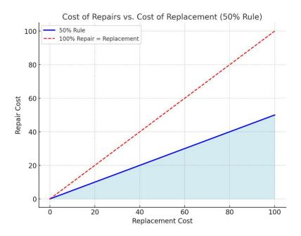
Here is the graph representing the cost of repairs versus the cost of replacement using the 50% rule. The blue line shows the 50% threshold, meaning if repair costs exceed this line (half of the replacement cost), replacement is advised. The red dashed line represents the point where repair costs equal replacement costs
